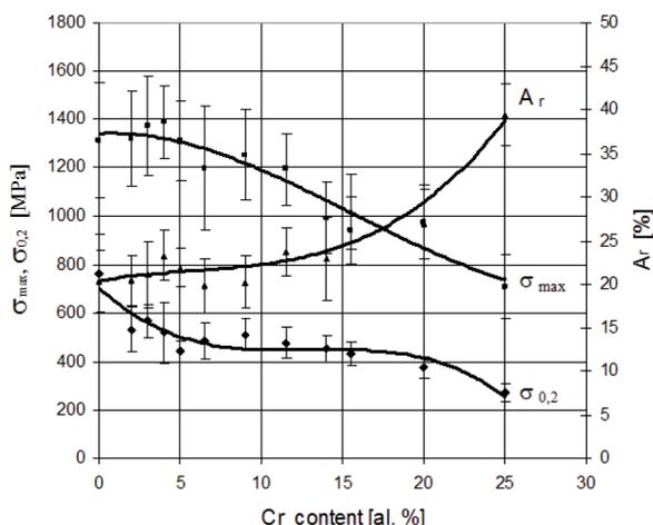
Fig. 6. Mechanical properties of the  $\text{Ni}_{75}\text{Al}_{(25-x)}\text{Cr}_x$  sinters at a room temperature
