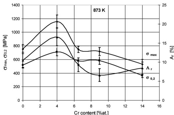
Fig. 8. Mechanical properties of the  $\text{Ni}_{75}\text{Al}_{(25-x)}\text{Cr}_x$  sinters at the temperature of 873K
