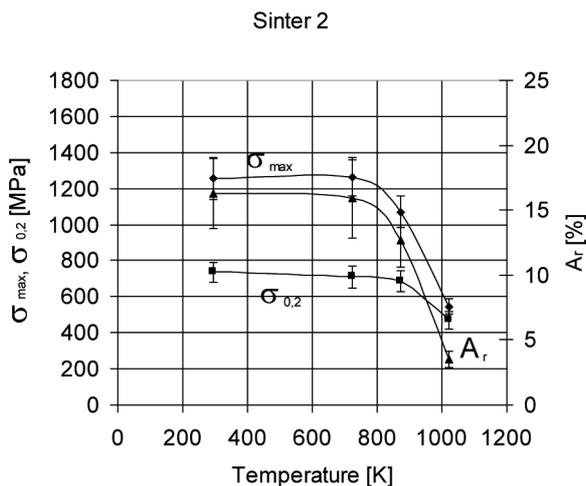
Fig. 12. Mechanical properties of a sinter obtained from: (80%) a mixture of Ni and Al powders (3:1 at.%) + (20%) mechanical synthesis product with the composition Ni<sub>75</sub>Al<sub>15</sub>Cr<sub>10</sub>
