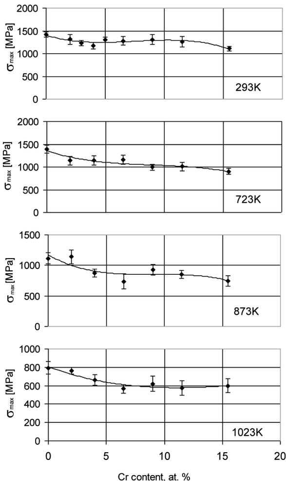
Fig. 2. The values of maximum true stress  $\sigma_{max}$  for the Ni<sub>75</sub>Al<sub>(25-x)</sub>Cr<sub>x</sub> alloys
