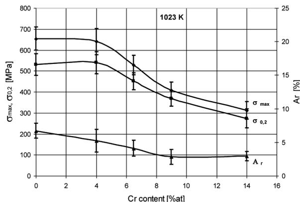
Fig. 9. Mechanical properties of the  $\text{Ni}_{75}\text{Al}_{(25-x)}\text{Cr}_x$  sinters at the temperature of 1023K
