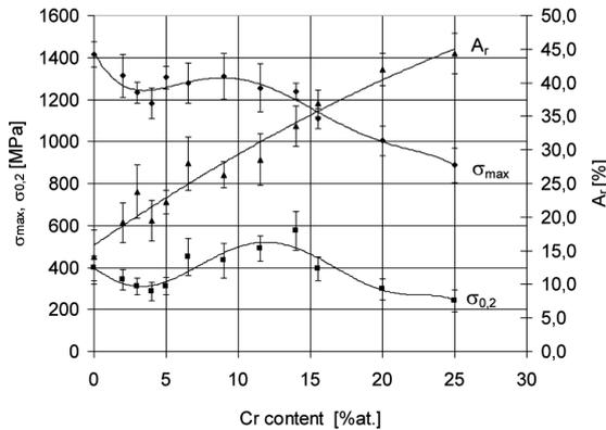
Fig. 1. Mechanical properties of the Ni<sub>75</sub>Al<sub>(25-x)</sub>Cr<sub>x</sub> alloys at room temperature
