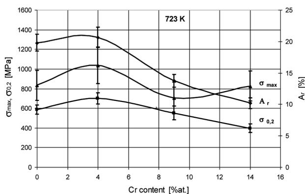
Fig. 7. Mechanical properties of the  $\text{Ni}_{75}\text{Al}_{(25-x)}\text{Cr}_x$  sinters at the temperature of 723K
