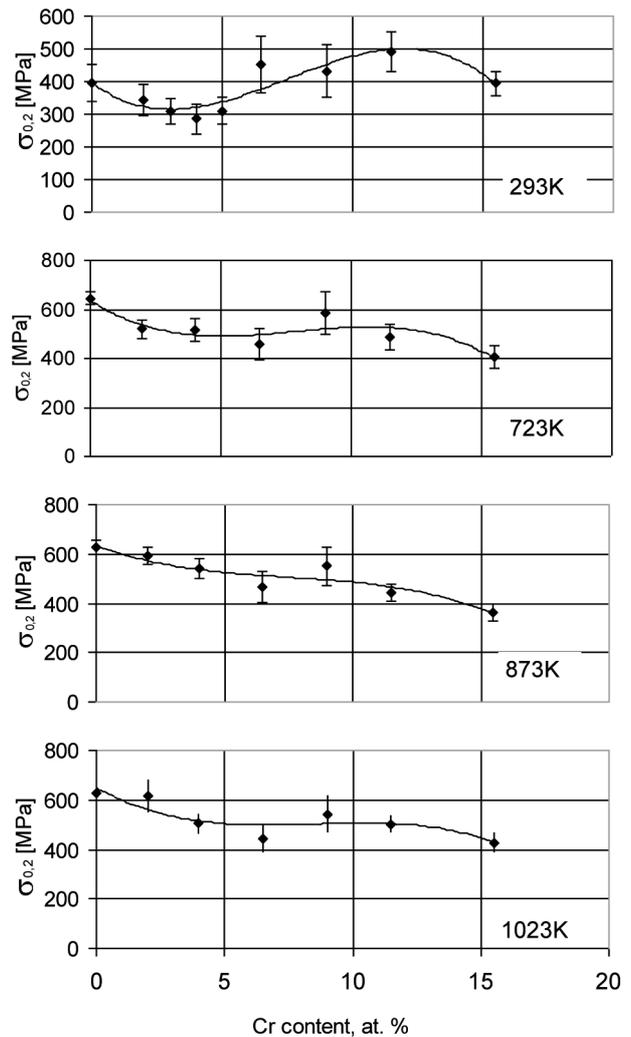
Fig. 3. The values of yield strength  $\sigma_{0.2}$  for the Ni<sub>75</sub>Al<sub>(25-x)</sub>Cr<sub>x</sub> alloys
