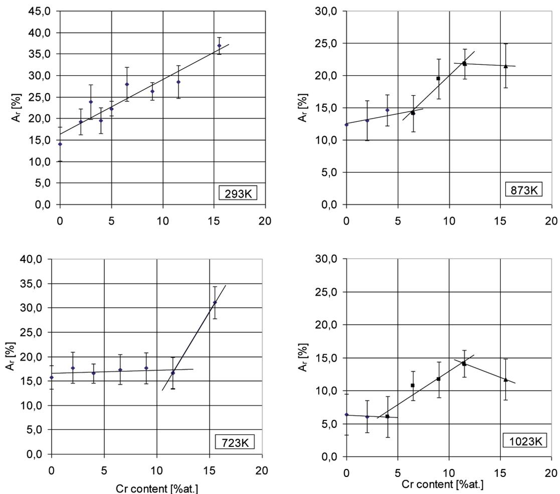
Fig. 4. The values of uniform contraction  $A_r$  for the Ni<sub>75</sub>Al<sub>(25-x)</sub>Cr<sub>x</sub> alloys
