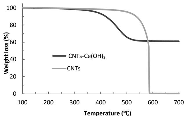
Fig. 3. TG curve of the  $\text{CeO}_2/\text{CNTs}$  precursor
