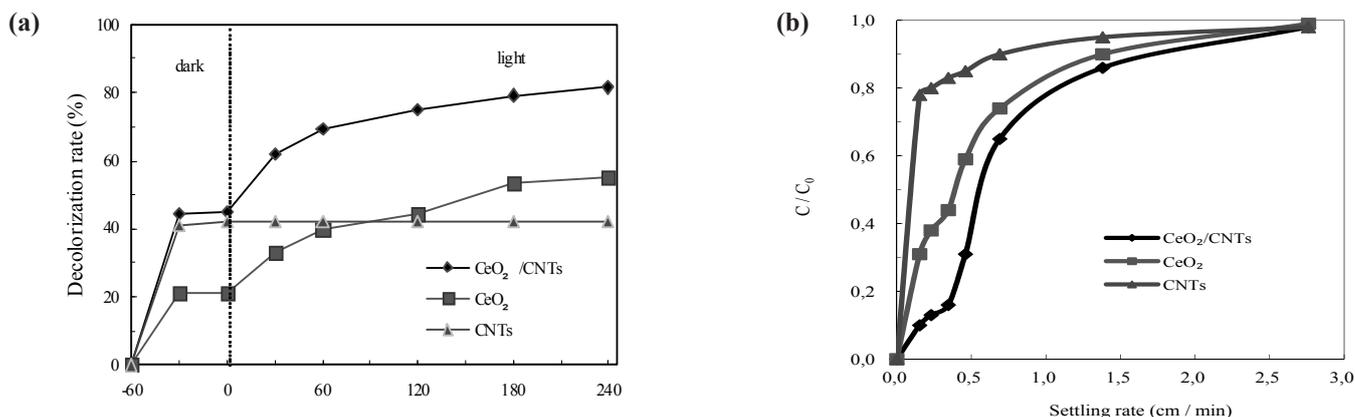
Fig. 6. Changes in the Acid Orange 7 concentration during dark adsorption and photocatalytic degradation (a) and sedimentation curves (b) in the presence of CeO<sub>2</sub>/CNTs, commercial CeO<sub>2</sub> and raw CNTs
