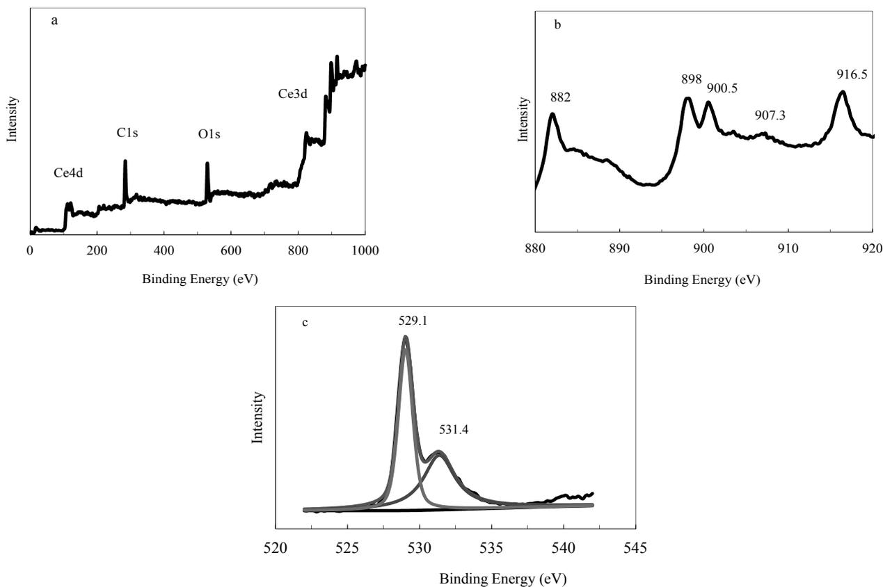
Fig. 5. XPS wide spectrum (a), Ce 3d spectrum (b) and O 1s spectrum (c) of CeO<sub>2</sub>/CNTs
