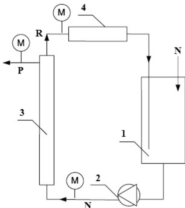
**Fig. 1.** Small-scale experimental rig: 1 – feed tank; 2 – pump; 3 – membrane module; 4 – radiator; N- feed water; R – retentate; P – permeate; M – manometer
