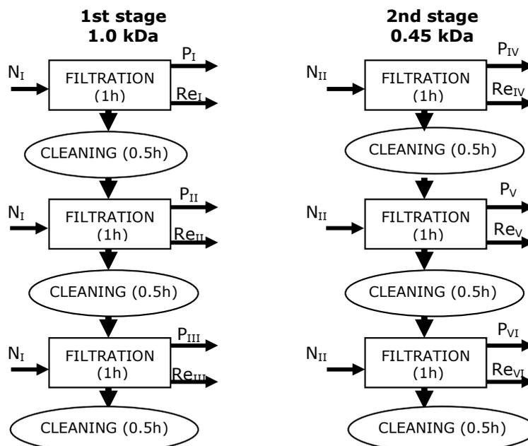
**Fig. 2.** A block diagram of the conducted experiment featuring the 1st and 2nd filtration stages.  $N_I$  – feed tank I (effluent water from RAS);  $N_{II}$  – feed tank II (mixed permeates  $P_I$ ,  $P_{II}$ ,  $P_{III}$  from the 1st filtration stage);  $Re_{I-VI}$  – retentates
