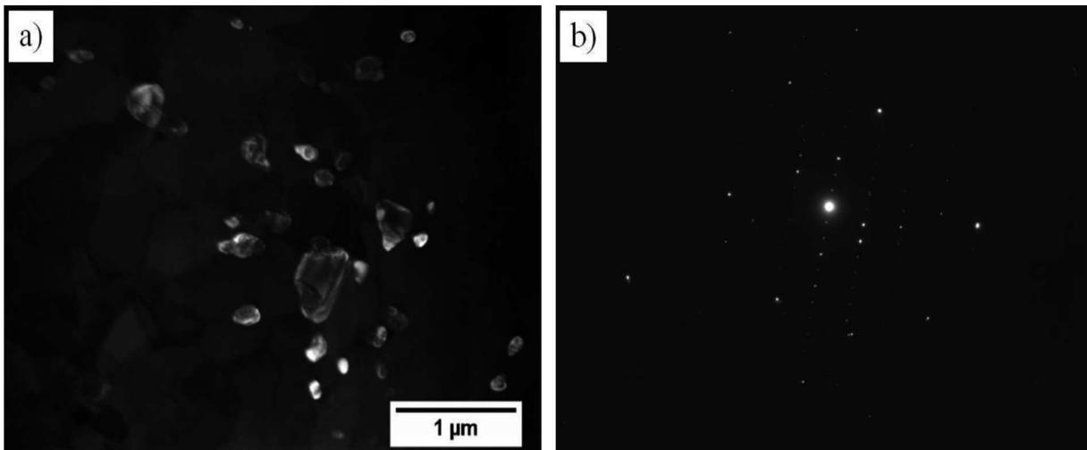
Fig. 2. Morphology of  $M_{23}C_6$  carbides in GP91 cast steel in the as-received condition, a) dark area from the reflection  $(4\bar{2}0)_{M_{23}C_6}$ ; b) electron diffraction pattern SAED,  $[1\bar{1}23]_{M_{23}C_6}$  and  $[3\bar{3}1]_{\alpha}$
