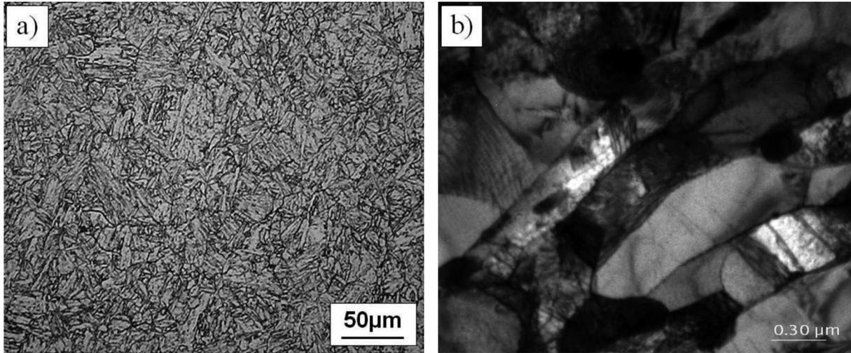
Fig. 1. Microstructure of GP91 cast steel in the as-received condition: a) OM, b) TEM
