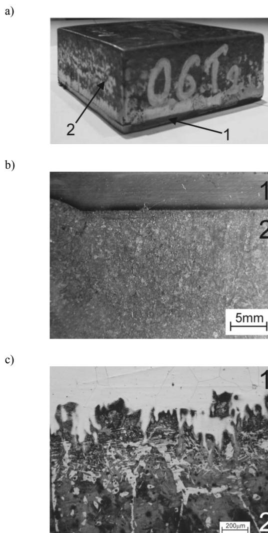
Fig. 3. View of test layered casting (a), its example traverse section (b) and microstructure of joint area (c): 1 – working part (layer) in form of alloy steel X2CrNi 18-9 plate, 2 – bearing part from unalloyed cast steel at carbon concentration  $C = 0,6\%$  and pouring temperature  $1650^{\circ}\text{C}$
