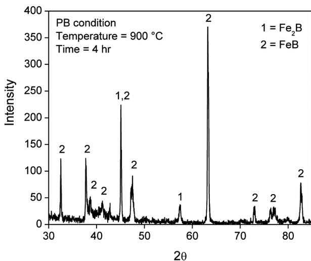
Fig. 2. X-ray diffraction patterns of the PB at a temperature of 900°C for about 4 hr
