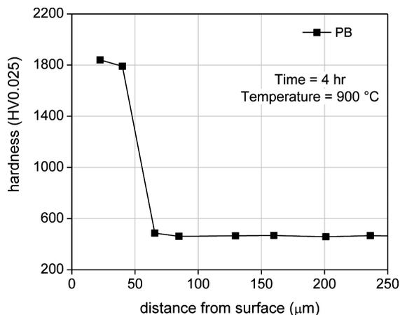
Fig. 4. Hardness depth profile of the PB at a temperature of 900°C for about 4 hr
