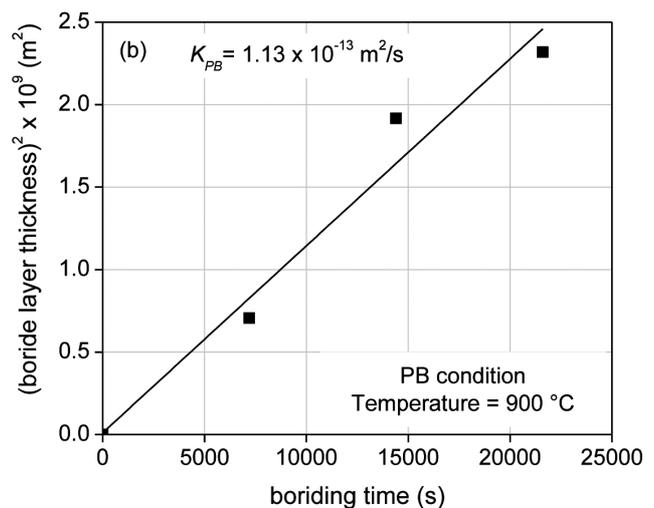
Fig. 3. The diagrams of (a) the boride layer thickness values and (b) square of the boride layer thickness values of the PB versus boriding time
