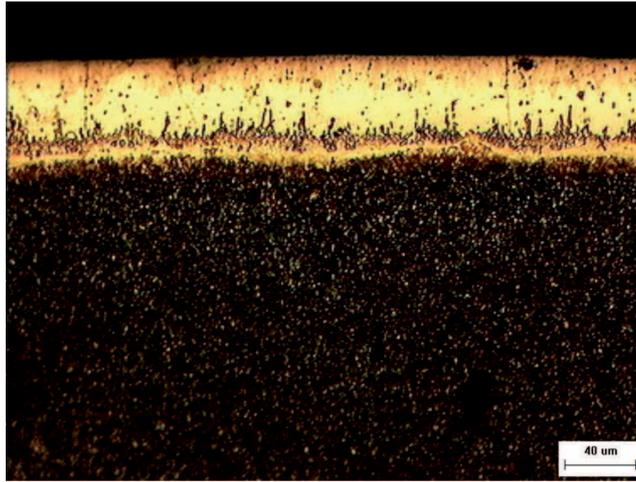
Fig. 1. The cross-sectional boride layer of the PB at a temperature of 900°C for about 4 hr
