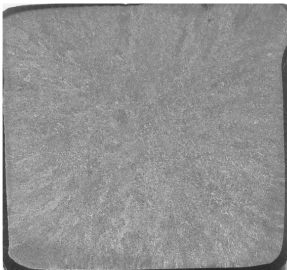
Fig. 2. Macrostructure of sample casting no 3_1
