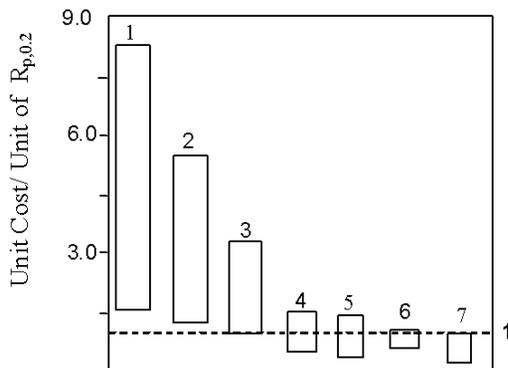
Fig. 2. Unit costs<sup>1</sup> of product essential for obtaining unit yield strength  $R_{p0.2}$  normalized towards forged steel (up to 1); (1) - aluminum alloys castings, (2) - forged aluminum, (3) - cast steel, (4) - forged steel, (5) - heat treated steel, (6) - ductile iron, (7) - ADI [1]
