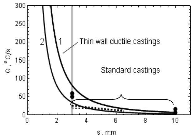
Fig. 3. Influence of wall thickness  $s$  and temperature  $T_i$  of liquid metal on the cooling rate of castings: line 1 - prediction for  $C=3.6\%$ ;  $Si=2.7\%$ ;  $T_i=1340^\circ C$ ,  $c=5.95 J/cm^3$ ,  $a=0.11 J/(cm^2 s^{1/2} ^\circ C)$ , line 2 - prediction for  $C=3.6\%$ ;  $Si=2.7\%$ ;  $c=5.95 J/cm^3$ ,  $T_i=1450^\circ C$ ,  $a=0.09 J/(cm^2 s^{1/2} ^\circ C)$  [4], points - experimental data [5], lines ----- experimental data [6]
