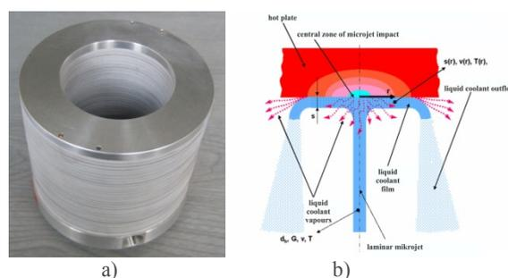
Fig. 3. Microjet device: a) general view of module, b) model of the zone of microjet impact against the plate surface
