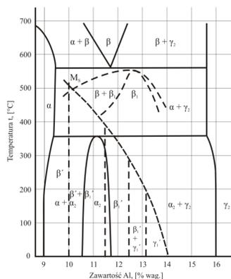
Fig. 7. Martensitic transformations in Cu-Al alloys [4]
