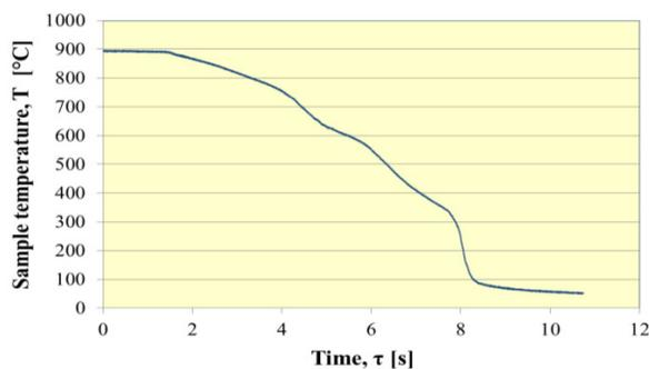
Fig. 5. Solution heat treatment curve in microjet cooling
