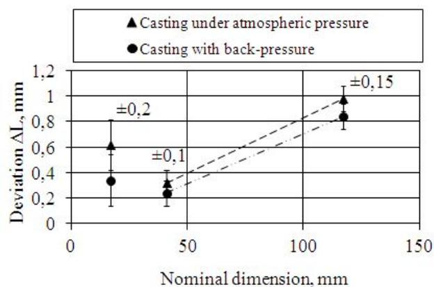
Fig. 6. Dimensional deviation  $\Delta L$  in function of the nominal dimension for casting from Fig. 7
