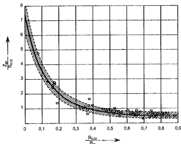
Fig. 1. Curve used in fatigue strength assessment [15]
