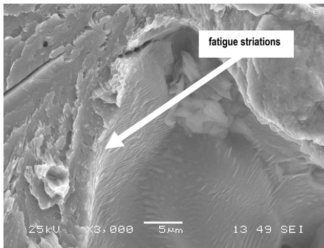
Ductile iron. Specimen 3, x3000, SEM.
