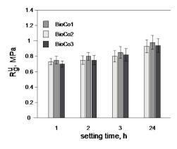
Fig. 1. Flexural strength measurement results for samples of sands bonded with BioCo binders hardened with Ca(OH)<sub>2</sub> and CO<sub>2</sub>
