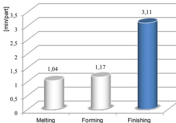
Fig. 3. Labour intensity for the chosen group of casts
