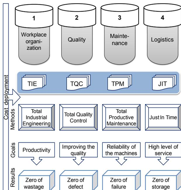
Fig. 1. Aims of production system improvement modules
