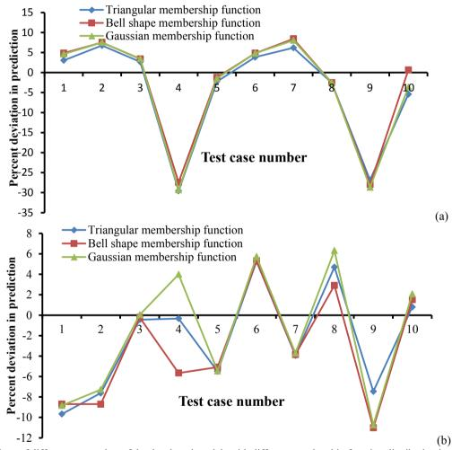
Fig 10 Comparison of different approaches of the developed models with different membership function distribution in terms of percent deviation in prediction for the response-SDAS, (a) Manually constructed fuzzy logic system and (b) Adaptive network based fuzzy logic system
