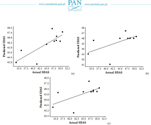
Fig 8 Comparison of predicted and actual SDAS via approach 1, (a) Triangular membership function distributions, (b) Bell shape membership function distributions and (c) Gaussian membership function distributions
