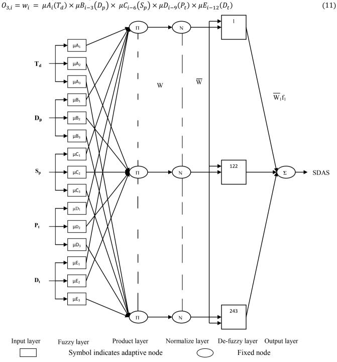
Fig. 6. ANFIS network architecture for predicting the response-SDAS
