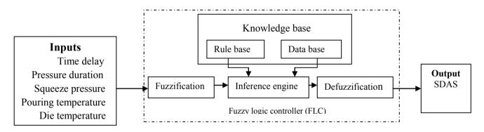
Fig. 3. Model representation of squeeze casting process using fuzzy interface system
