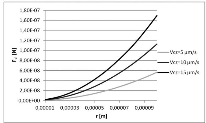
Fig. 4. Results of calculations of drag force  $F_d$  depending on the radius of  $\text{Al}_2\text{O}_3$  particle in the vicinity of solidification front vertically moving at a rate of  $V=5$   $\mu\text{m/s}$ ,  $10$   $\mu\text{m/s}$  and  $15$   $\mu\text{m/s}$
