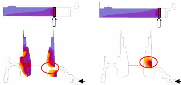
Fig. 8. Simulation results of air entrapment phenomena corresponding to chosen stages of piston positions in shot sleeve. a – in shot sleeve from beginning to final piston position, b – two chosen stages (70 step and 89 step) connecting the piston position with air entrapment map inside of casting (for different piston speed)
