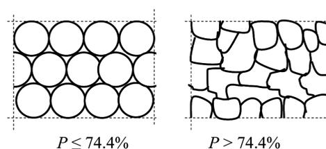
Fig. 1. Relation between porosity and bubble shape [4]
