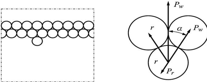
Fig. 2. Distribution of forces between foam bubbles [4]
