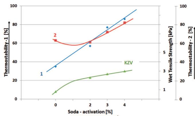
Fig. 3. Thermostability of the Slovak bentonite *Bentovet K* (measured by a method through the compression strength – 1); measured through the wet tensile strength – 2) in dependence on the Soda – activation degree)
