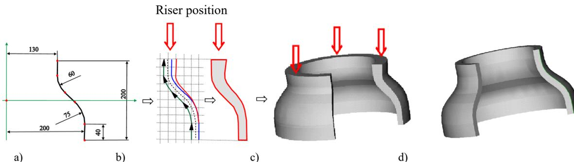
Fig. 3. Design of the casting using the module "CastDesigner" based on the "track curve"
