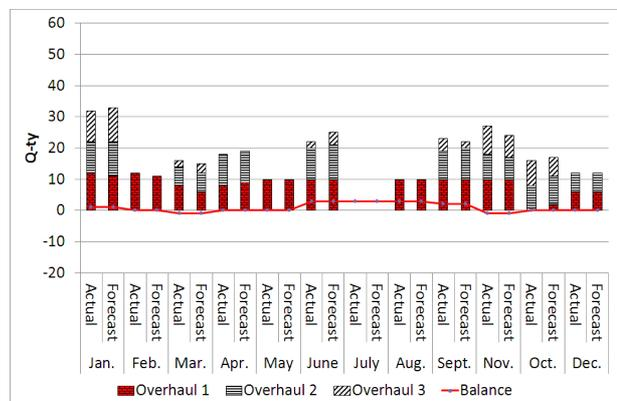
Fig. 7. Execution of forecast (ANN model) for spare bearing P/N 88.06.3276.
