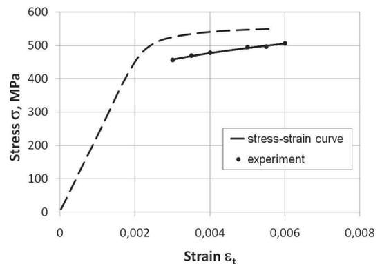
Fig. 7. Cyclic strain graph of steel P91
