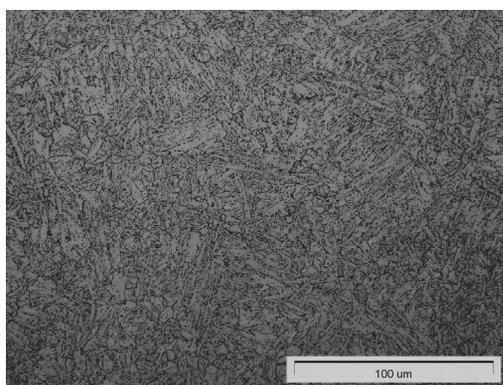
Fig. 1. Microstructure of P91 steel, LM
