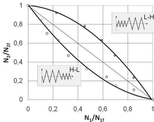
Fig. 16. Characteristics of the low-cycle fatigue durability of P92 steel under graded loads
