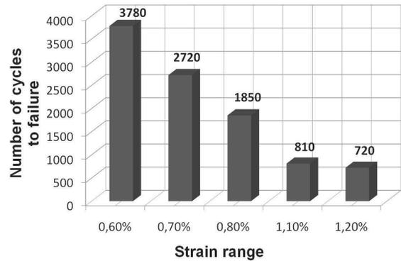
Fig. 5. Low-cycle fatigue of P91 steel
