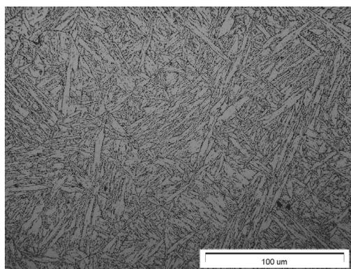
Fig. 2. Microstructure of P92 steel, LM
