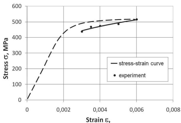
Fig. 8. Cyclic strain graph of P92 steel
