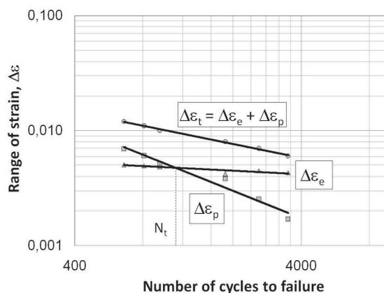
Fig. 11. Fatigue durability graphs of P91 steel
