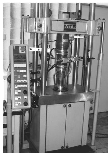
Fig. 4. Servohydraulic test system MTS-810
