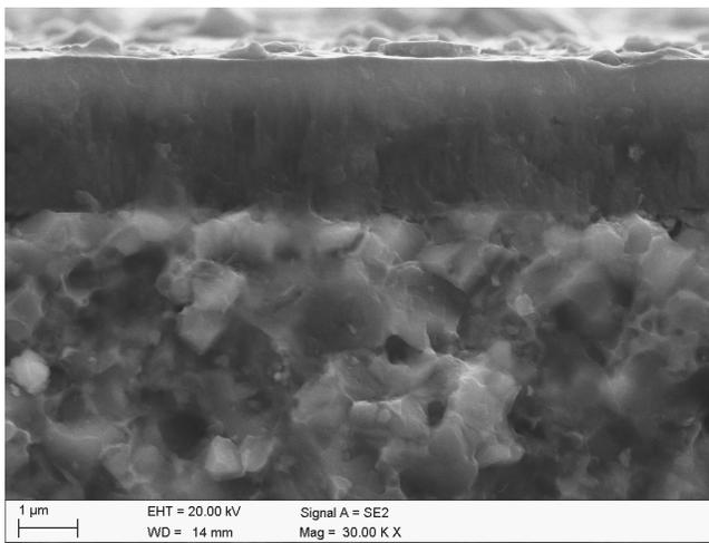
Fig. 4. Fracture surface of the gradient Ti(C,N) coating deposited onto the cermet substrate
