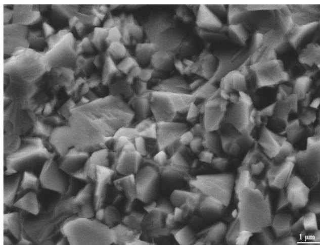
Fig. 2. Structure from the cemented carbides
