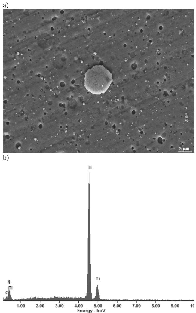
Fig. 6. a) Surface topography of the gradient Ti(C,N) coating deposited onto the cermet substrate and b) X-ray energy dispersive plot the area X
