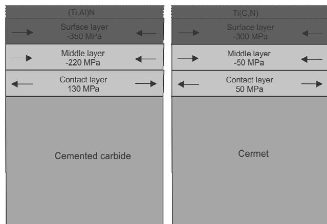
Fig. 13. Schematic distribution of stresses in the gradient coating (Ti,Al)N and Ti(C,N) deposited on cemented carbide and cermet substrate obtained by computer simulation
