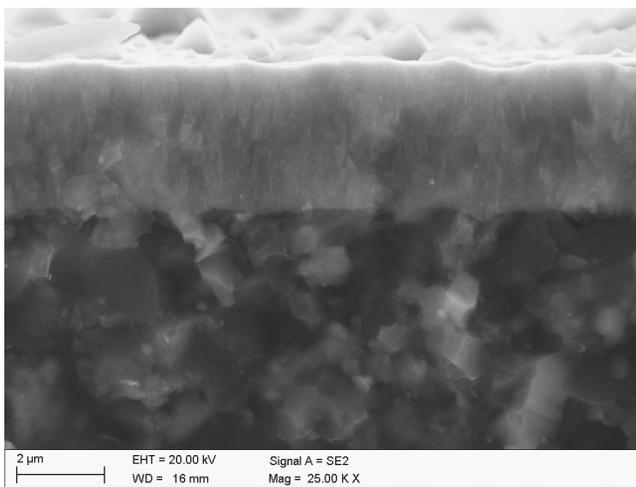
Fig. 5. Fracture surface of the gradient (Ti,Al)N coating deposited onto the  $\text{Al}_2\text{O}_3+\text{TiC}$  oxide tool ceramics substrate
