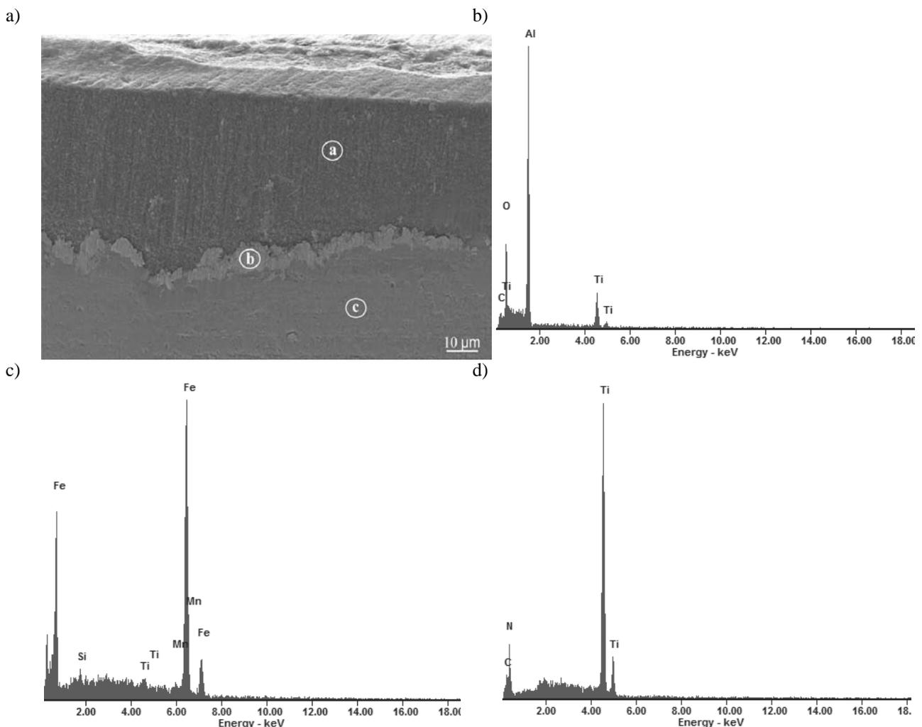
Fig. 12. a) Character of wear of the Al<sub>2</sub>O<sub>3</sub>+TiC oxide tool ceramics sample with Ti(C,N) coating, investigated with SEM, b) X-ray energy dispersive spectrum from the area "a" on figure a), c) X-ray energy dispersive spectrum from the area "b" on figure a), d) X-ray energy dispersive spectrum from the area "c" on figure a)
