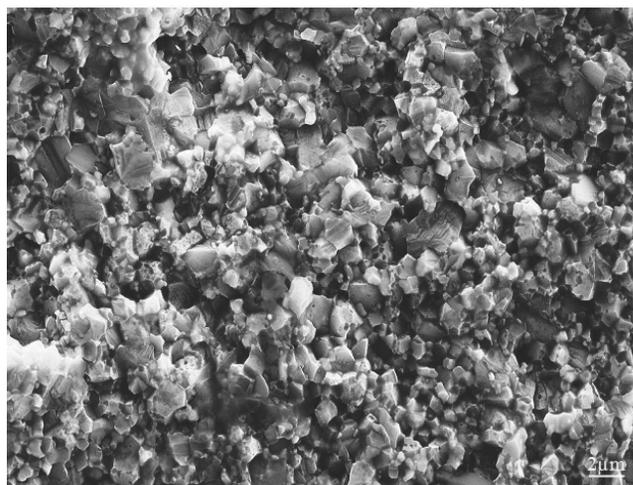
Fig. 3. Structure from the oxide ceramics  $\text{Al}_2\text{O}_3+\text{TiC}$
