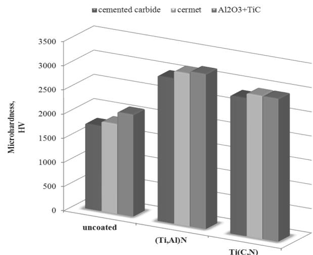
Fig. 10. Comparison of the microhardness of the investigated materials
