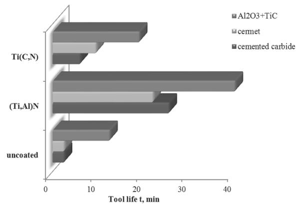
Fig. 11. Comparison of tool life for tools from cemented carbides, cermets and oxide ceramics with gradient (Ti,Al)N and Ti(C,N) type coatings with uncoated tool
