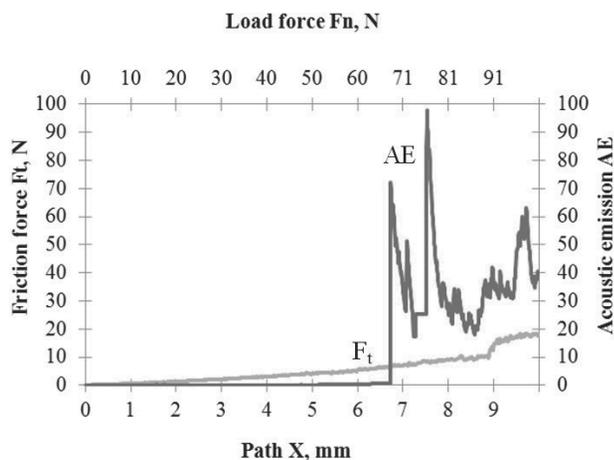
Fig. 8. Diagram of the dependence of the acoustic emission (AE) and friction force  $F_t$  on the load for the  $\text{Al}_2\text{O}_3+\text{TiC}$  oxide tool ceramics with the (Ti,Al)N coating
