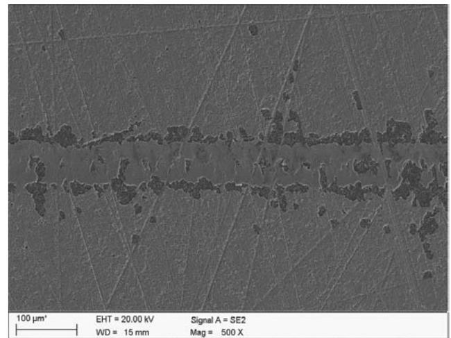
Fig. 9. Characteristic failure obtained by scratch test of the Ti(C,N) coating deposited on  $\text{Al}_2\text{O}_3+\text{TiC}$  oxide tool ceramics
