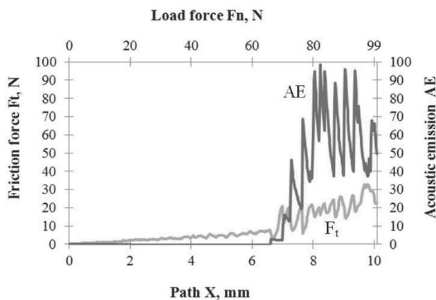
Fig. 7. Diagram of the dependence of the acoustic emission (AE) and friction force  $F_t$  on the load for the cemented carbide with the Ti(C,N) coating
