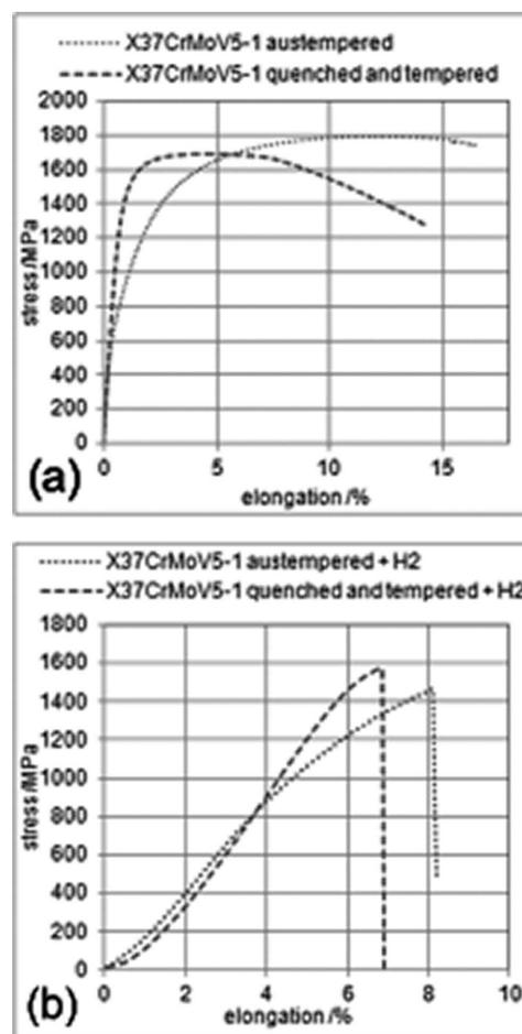
Fig. 3. Tensile curves of the X37CrMoV5-1 steel after austempering and quenching and tempering treatments before (a) and after (b) hydrogen charging
