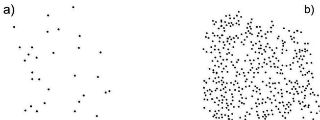
Fig. 4. Examples for the distribution of voids in bulk solders at High  $T_{PEAK}$  (in binary images); (a) galvanic Sn; (b) immersion Sn
