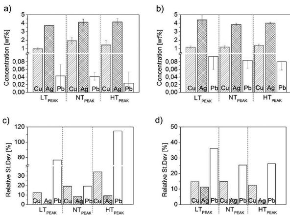
Fig. 1. Measured concentrations of Cu; Ag and Pb elements at galvanic Sn (a; c) and immersion Sn (b; d),  $LT_{PEAK}$  = Low  $T_{PEAK}$ ,  $NT_{PEAK}$  = Normal  $T_{PEAK}$ ,  $HT_{PEAK}$  = High  $T_{PEAK}$
