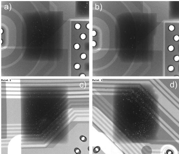
Fig. 3. Characteristics of voids [area fraction; count number; maximum diameter] in bulk solders for cases of galvanic Sn (a; b) and immersion Sn (c; d); (a)  $LT_{PEAK}$  [2.4%, 69 pcs,  $d_{max} = 22 \mu m$ ]; (b)  $HT_{PEAK}$  [1.3%, 30 pcs,  $d_{max} = 22 \mu m$ ]; (c)  $LT_{PEAK}$  [4.6%, 255 pcs,  $d_{max} = 24 \mu m$ ]; (d)  $HT_{PEAK}$  [7.1%, 333 pcs,  $d_{max} = 28 \mu m$ ]
