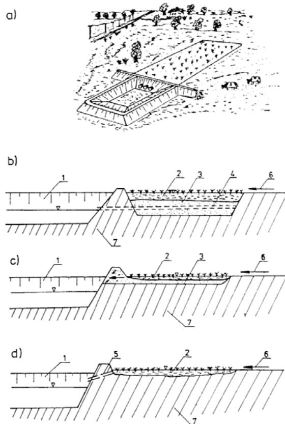
Fig. 7. A scheme of reservoir for preliminary surface runoff water purification: a) general view of the reservoir, b), c), d) cross sections of different types of reservoirs of verified construction; 1 – pond, 2 – initial pond (biofilter) of 20–30 cm depth covered by plants, 3 – filtration material (sand), 4 – drainage, 5 – pipeline draining water (or space in the crown of the dike), 6 – water flow direction, 7 – poorly permeable substratum
