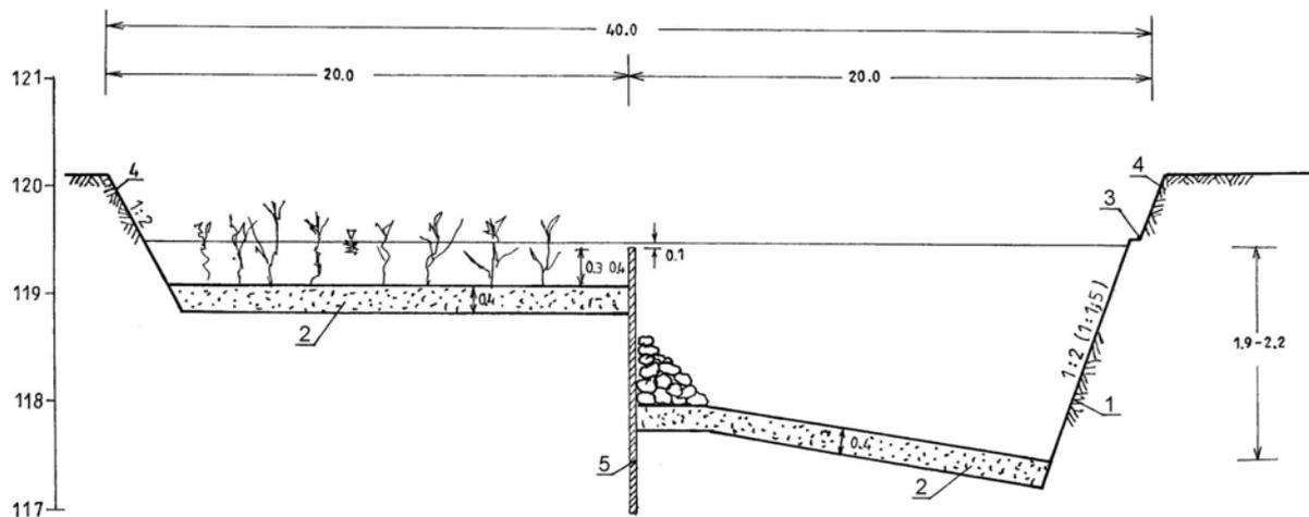
Fig. 4. A schematic cross section through the natural swimming pool; 1 – slope of the deep part of the pool, 2 – bottom (gravel, coarse sand), 3 – bench allowing a walk over the water table, 4 – slope covered by grass, 5 – wall separating the deep part of the pool from the shallow one
