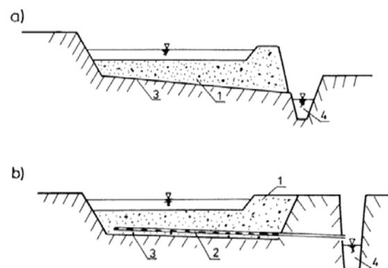
Fig. 10. Schemes of filtration basins: a) simple basin, b) drained basin; 1 – filtration material, 2 – drainage with a filter cover, 3 – natural bottom (impermeable or poorly permeable) or sealed with plastic, 4 – infiltrating water recipient (water course, pond, channel, pipeline, etc.)
