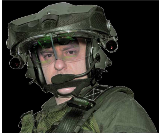
Fig. 16. Tales TopOwl® helmet incorporate an optical combiner assembly for each eye, allowing the pilot to view the cockpit and the outside world directly with the night imagery superimposed on it. TopOwl® has a 40° FOV and a total headborne weight of 2.2 kg in full configuration. Reproduced from [16].
