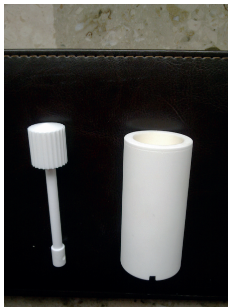
Fig. 2. Photograph of measurement tools (material - alumina) used in investigations
