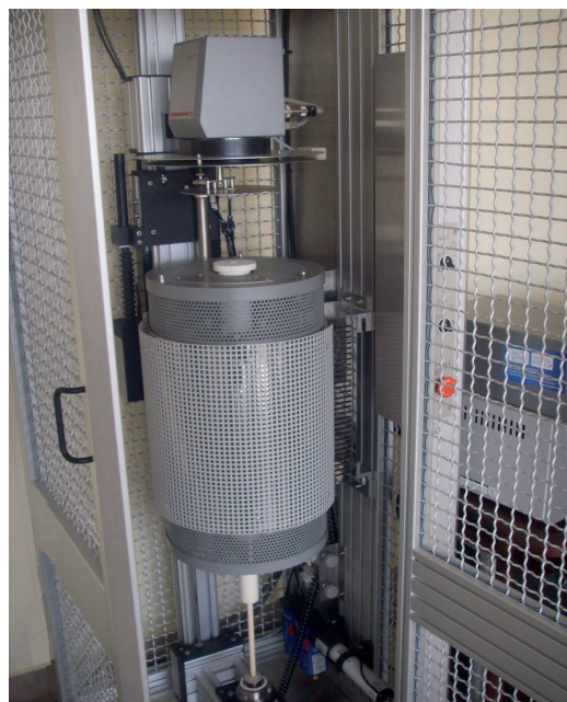
Fig. 3. Photograph of rotational viscometer used in investigations
