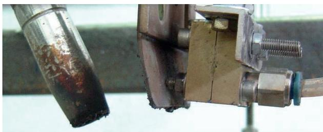
Fig. 3. Montage of welding head and micro-jet injector
