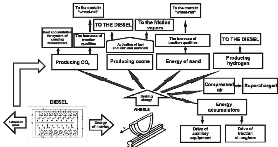
Fig. 1. The locomotive scheme with rational use of the braking energy
