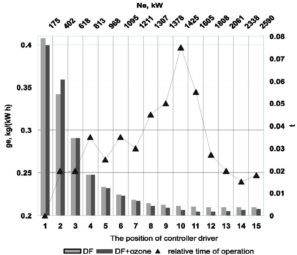
Fig. 3. Changes in specific fuel efficiency for diesel 16GHN 26/26 of locomotive 2TE116U in operation according to the diesel characteristic
