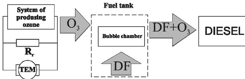
Fig. 2. The scheme of use of the energy of electrodynamic braking for obtaining ozone with further ozonized fuel
