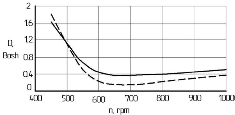
Fig. 4. The change of the exhaust opacity at operation according to the locomotive characteristic of diesel 16GHN 26/26 of locomotive 2TE116U
