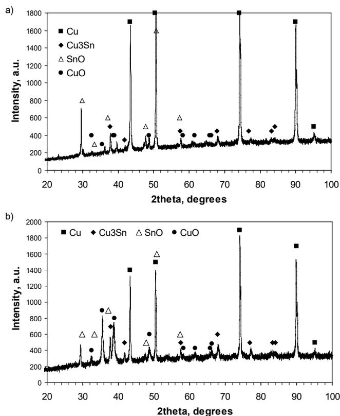
Fig. 4. Diffraction pattern of tin stripped copper substrate in solutions: a) 2M NaOH + 3% H<sub>2</sub>O<sub>2</sub>, b) 2M NaOH + 3% (NH<sub>4</sub>)<sub>2</sub>S<sub>2</sub>O<sub>8</sub>
