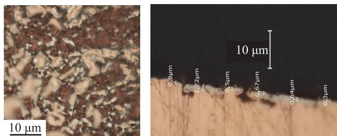
Fig. 5. Surface and cross-section of the samples after tin stripping in 2M NaOH + 3% H<sub>2</sub>O<sub>2</sub> solution for 20 min (80 °C)
