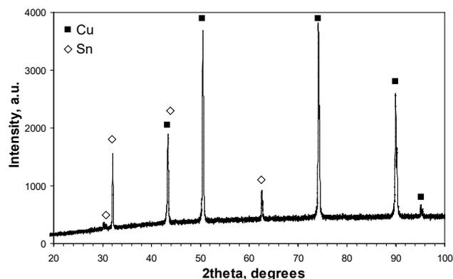
Fig. 2. Diffraction pattern of tin coated copper substrate
