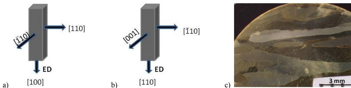
Fig. 1. Samples before the deformation process: schematic representation of the orientation of single crystals a) and b), and microstructure of polycrystalline Cu-8.5% at. Al alloy on a surface perpendicular to the extrusion direction c)
