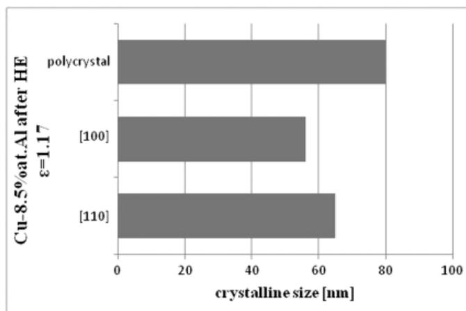
Fig. 4. Crystalline size of samples after HE  $\varepsilon = 1.17$
