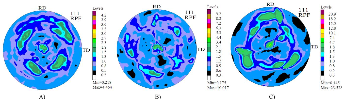
Fig. 6.  $\{111\}$  pole figures for Cu-8.5%at. Al single crystals after the hydrostatic extrusion process, with initial orientations of A)  $\langle 110 \rangle$ , B)  $\langle 100 \rangle$ , and C) polycrystal
