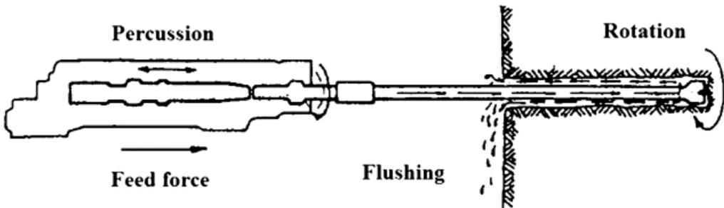
Fig. 1. A typical Top Hammer drill (Jimeno, 1995)
