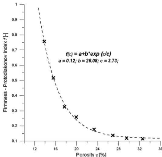
Fig. 4. The  $f$ - $\varepsilon$  relation for examined briquettes
