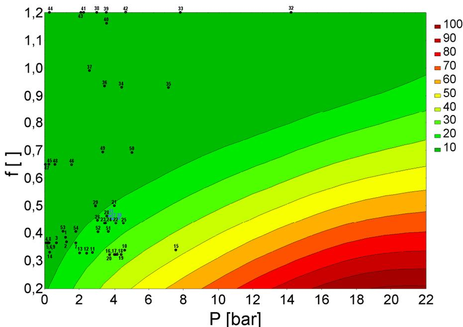
Fig. 7. In situ measurements and laboratory outburst risk
