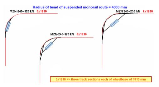
Fig. 19. Kinematics of modular load-carrying systems on a bend
