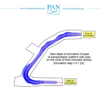
Fig. 12. Exemplary simulation test. Next steps of simulation of pass of transportation platform with load on route of floor-mounted railway
