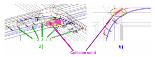
Fig. 32. Simulation of transportation of powered-roof support by MZN-252-252kN modular load-carrying system on a route bend: a) next selected steps of simulation of bend overcoming, b) exemplary simulation step – collision solid of support and belt conveyer – top view
