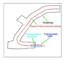
Fig. 10. Components of simulation model - drawing documentation
