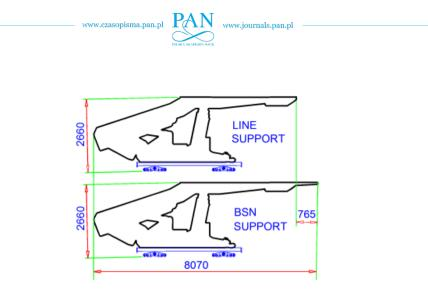
Fig. 8. Load transported by floor-mounted railway - external outline
