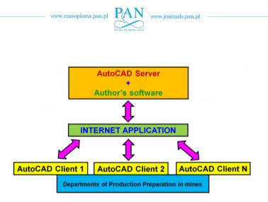
Fig. 3. Concept of the system for collision analyses on transportation routes
