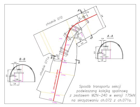
Fig. 2. Example of present testing the collision during transportation by suspended monorail. The drawing made by KWK Ziemowit mine is a part of transportation documentation
