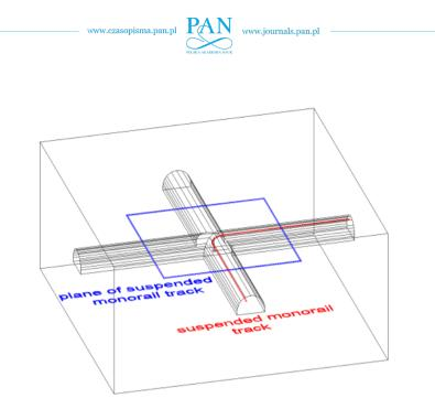
Fig. 24. Suspended monorail track in relation to solid model of the roadway
