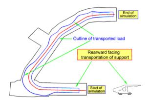
Fig. 13. Exemplary simulation. Determination of outline of transported load. Rearward facing transportation of the support
