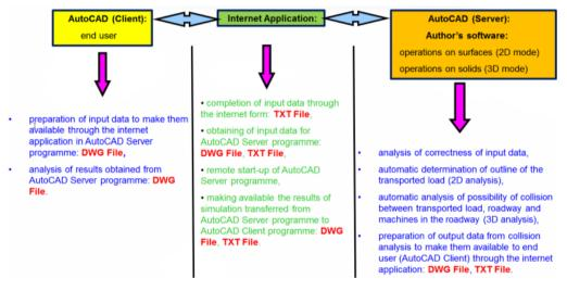
Fig. 4. Structure of Client - Server application for collision analyses on transportation routes
