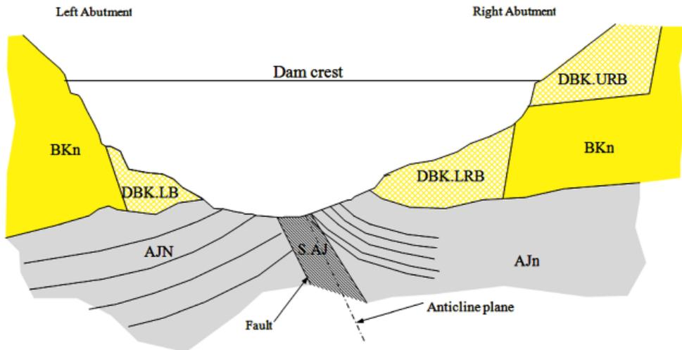
Fig. 2. Geological cross-section of Gotvand Olya dam
