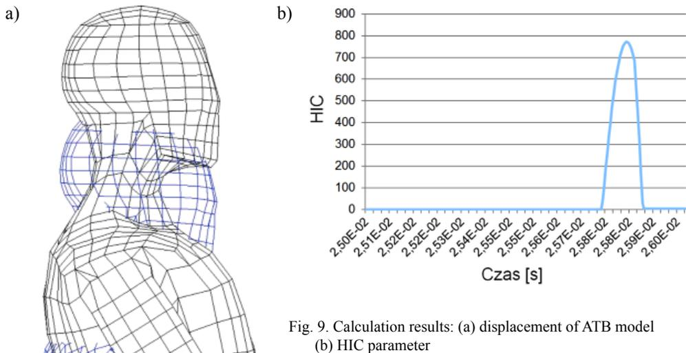
Fig. 9. Calculation results: (a) displacement of ATB model
