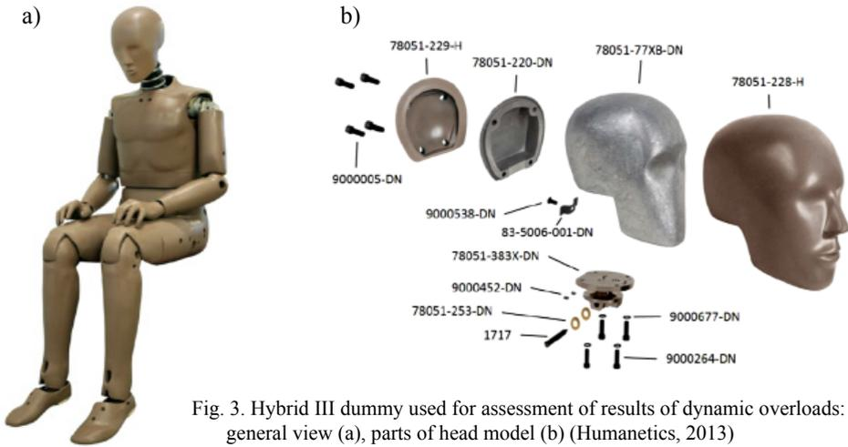
Fig. 3. Hybrid III dummy used for assessment of results of dynamic overloads: general view (a), parts of head model (b) (Humanetics, 2013)
