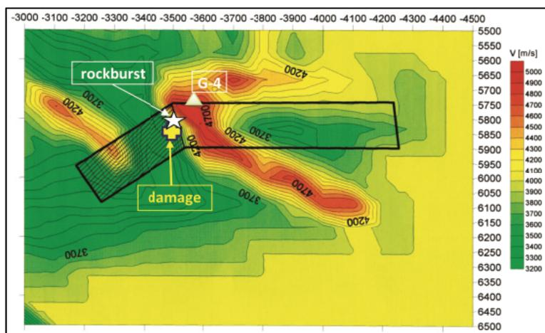
Fig. 3. Bobre mine, coal panel no 6/510. Tomographic velocity image (m/s) calculated from seismic events recorded between June 15<sup>th</sup> 2011 and July 15<sup>th</sup> 2011. The star mark shows the epicenter of strong seismic tremor with seismic energy  $E = 8 \cdot 10^6$  J; the cross mark depicts location of damaged mine workings due to rock burst in coal seam
