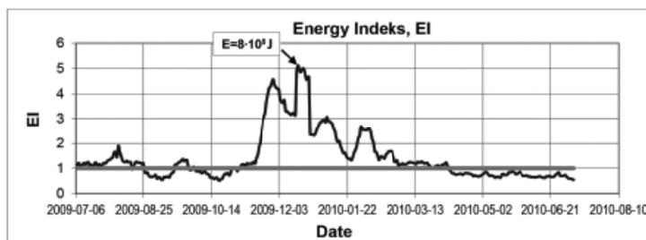
Fig. 2. An example of sequential distribution of  $EI$  parameter in moving time windows with the progress of 1 day in coal panel no. 3/503. On December 16, 2009 the strongest tremor of seismic energy  $E = 8 \cdot 10^8 \text{ J}$  ( $M_L = 3.7$ ) occurred at a time when was the highest value of  $EI$  parameter
