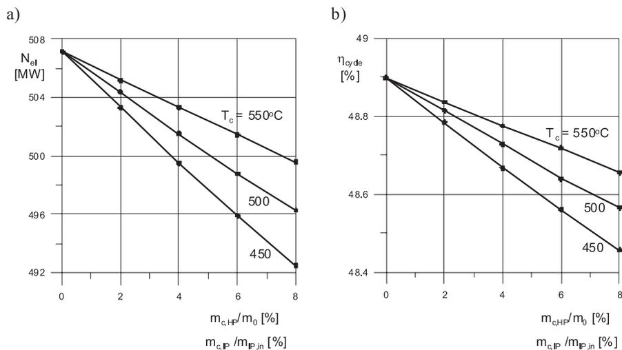
Figure 13. Combined effect of the HP and IP cooling system.
