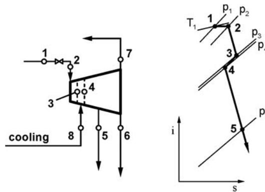
Figure 5. Mixing process.
