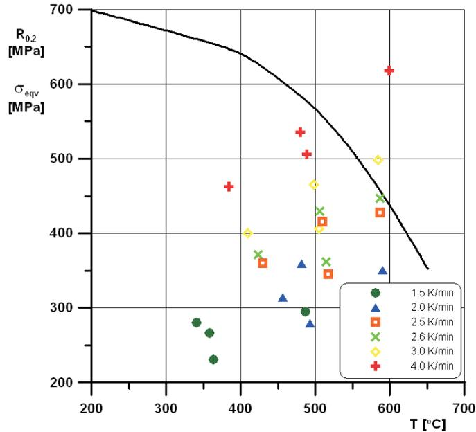
Figure 18. Values of maximum von Mises stress for different increment rates  $\Delta T/\Delta t$  during start-up compared to the yield stress (points – maximum values of equivalent (von Mises) stress in start-ups, curve – yield stress  $R_{0.2}$ ).
