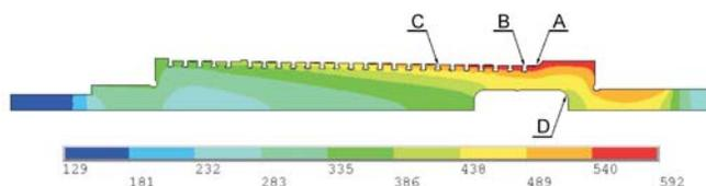
Figure 12. Temperature distribution in the rotor of the turbine HP part in the 106th minute of the start-up process.
