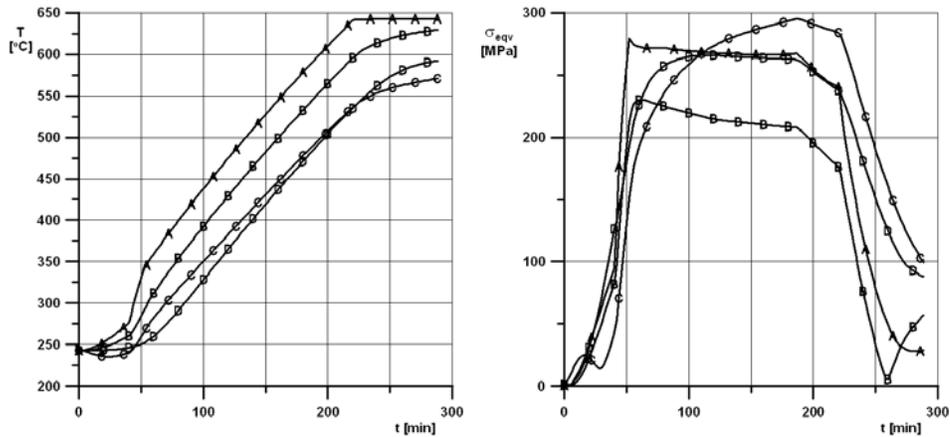
Figure 7. Curves illustrating changes in the metal temperatures and in the equivalent (von Mises) stress in the critical areas of the rotor of the turbine HP part for  $\Delta T/\Delta t = 1.5$  K/min.
