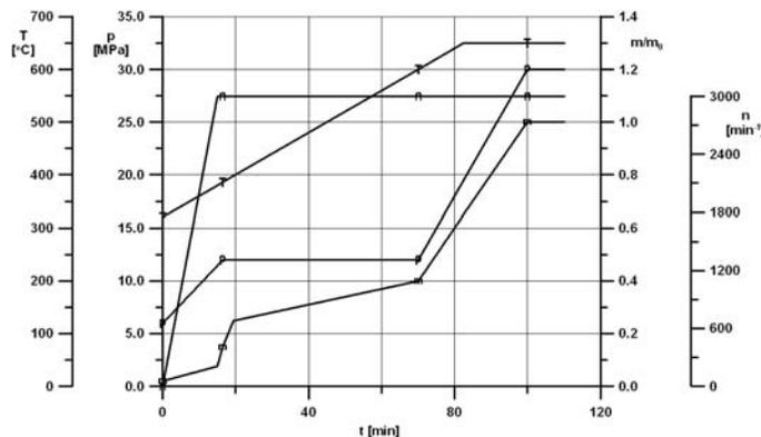
Figure 5. Power unit start-up curve from initial cold state for the live steam temperature increment  $\Delta T/\Delta t = 4.0 \text{ K/min}$  ( $T$  – live steam temperature,  $p$  – live steam pressure,  $n$  – rotor revolutions,  $m/m_o$  – turbine feed steam mass flow to the nominal steam mass flow ratio).
