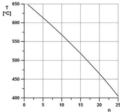
Figure 3. Change in steam temperature along the flow system of the turbine HP part ( $n$  – number of stage).
