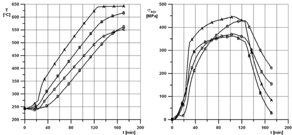
Figure 11. Curves illustrating changes in the metal temperatures and in the equivalent (von Mises) stress in the critical areas of the rotor of the turbine HP part for  $\Delta T/\Delta t = 2.6$  K/min.
