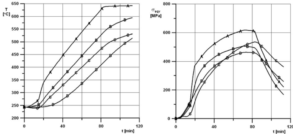
Figure 6. Curves illustrating changes in the metal temperatures and in the equivalent (von Mises) stress in the critical areas of the rotor of the turbine HP part for  $\Delta T/\Delta t = 4.0$  K/min (A – first thermal groove, B – bottom land of the first blade groove, C – bottom land of the seventh blade groove, D – corner of the internal chamber).
