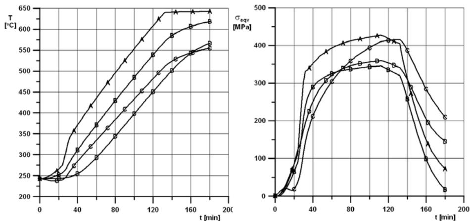
Figure 10. Curves illustrating changes in the metal temperatures and in the equivalent (von Mises) stress in the critical areas of the rotor of the turbine HP part for  $\Delta T/\Delta t = 2.5 \text{ K/min}$ .
