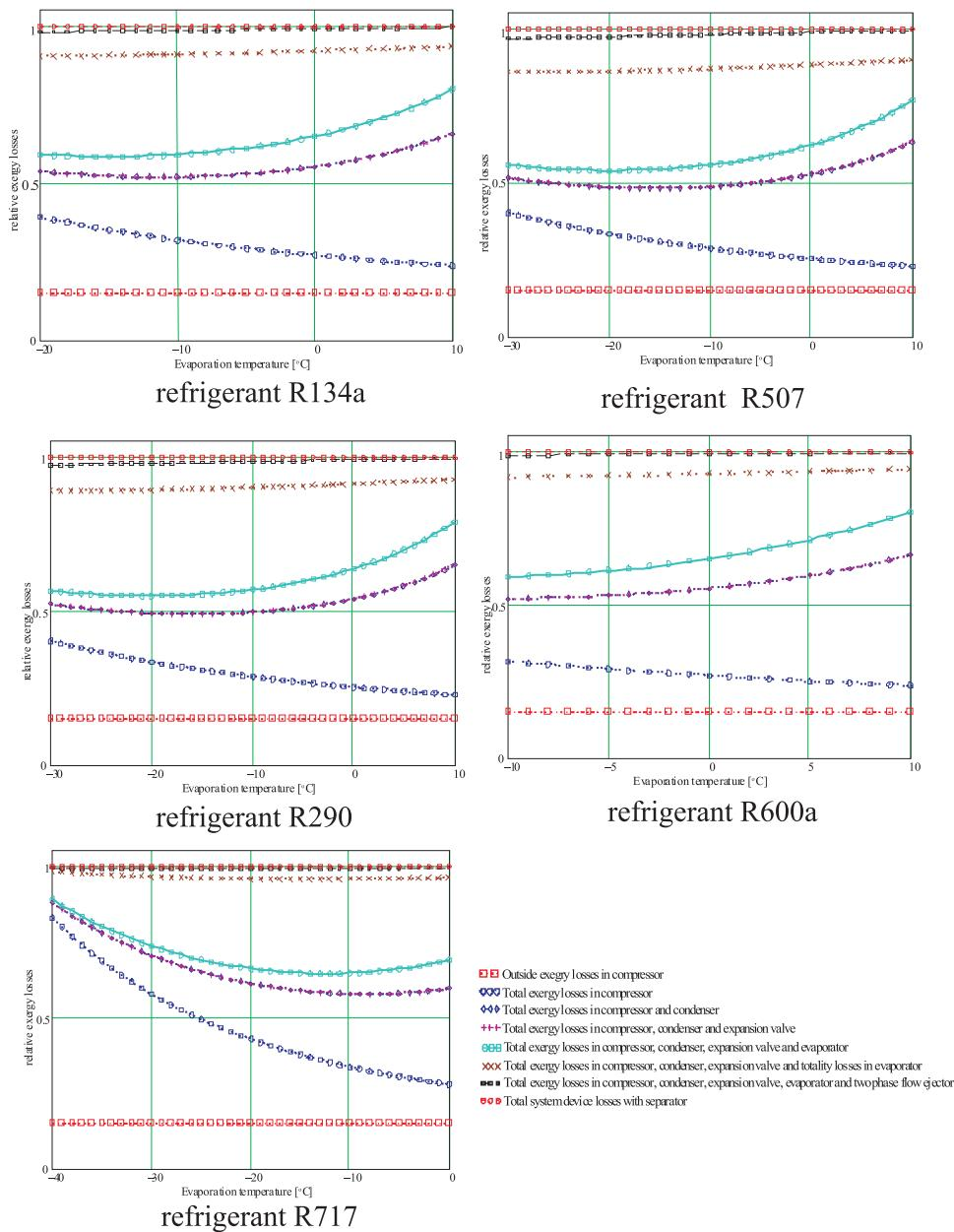
Figure 5. Relative exergy losses of ejector-compression refrigeration cycle vs. temperature of evaporation at condensation temperature  $t_k = 35^\circ\text{C}$  for various working fluids.
