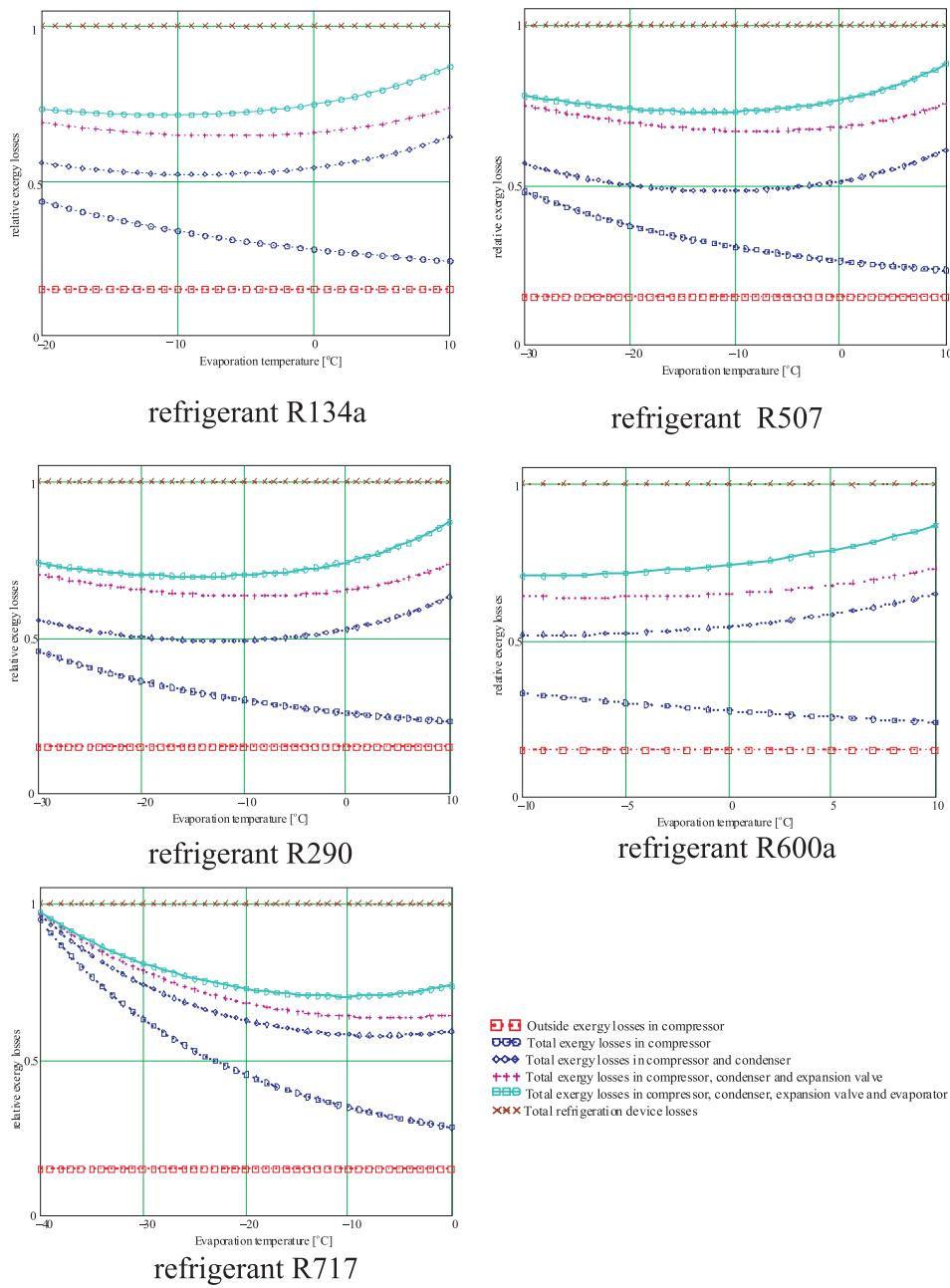
Figure 4. Relative exergy losses of compression refrigeration cycle vs. temperature of evaporation at condensation temperature  $t_k = 35^\circ\text{C}$  for various working fluids.
