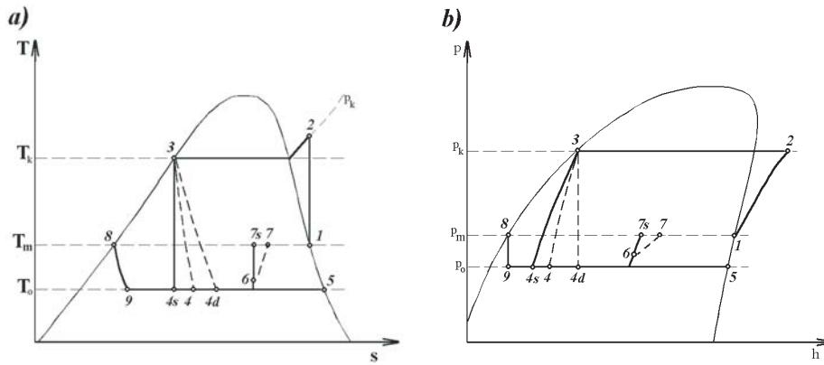
Figure 2. Thermodynamic cycles of ejector-compression system: a) at  $T$ - $s$  coordinates, b) at  $p$ - $h$  coordinates.
