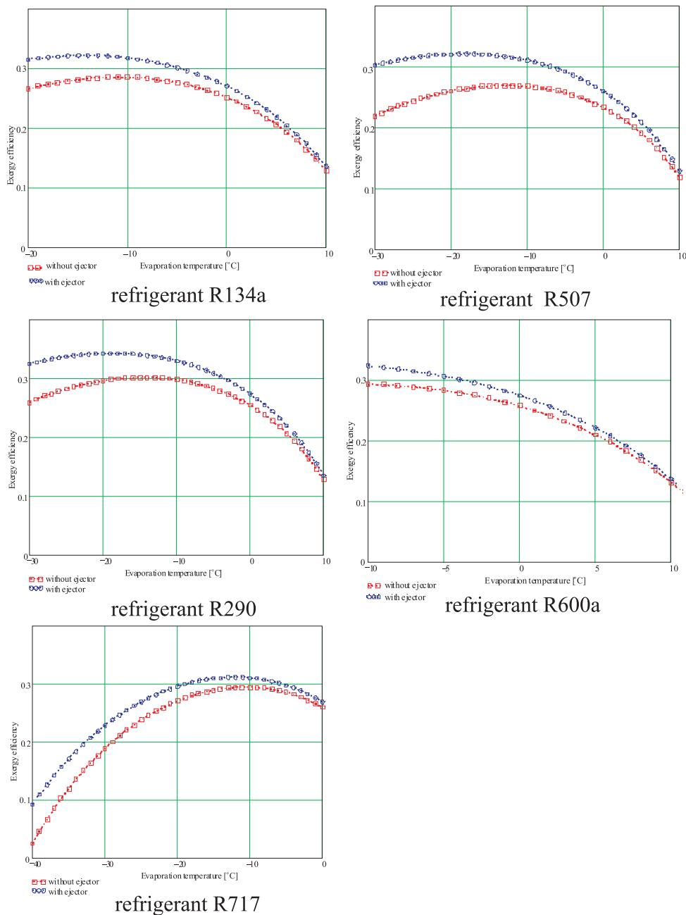
Figure 6. Exergy efficiency vs. temperature of evaporation of ejector-compression and compression refrigeration cycles at condensation temperature  $t_k = 35$  °C for various working fluids.
