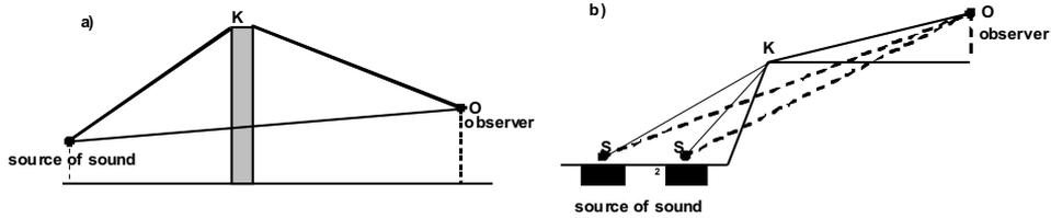
Fig. 2. Scheme of diffraction of acoustic wave encountering an obstacle
