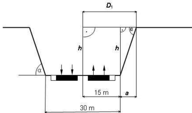
Fig. 1. Scheme of cross-section of motorway A2 section Komorniki - Krzesiny
