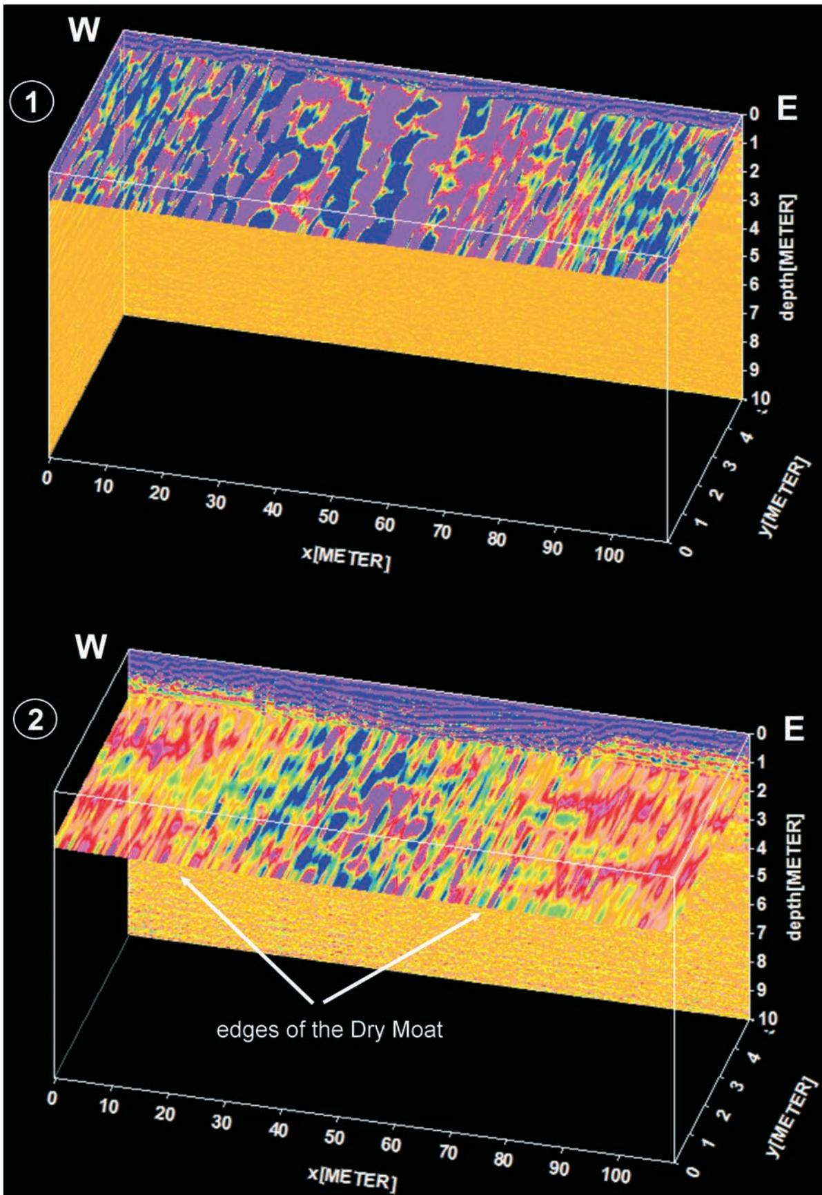
**Fig. 10.** GPR quasi-3D block-diagrams (slices) of the western section of the Dry Moat. 1: upper part of aeolian filling. 2: lower part of aeolian sediments with marked edges of DM. Processed by F. Welc.
