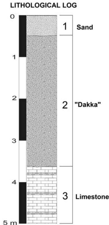
**Fig. 8.** Synthetic lithological log for west Saqqara area. 1 – wind-blown eolian sands, 2 – calcareous debris cemented with calcium carbonate with a sandy-clay-silty matrix, so-called *dakka*, 3 – erosional top of Paleogene limestones. Drawn by F. Welc.
