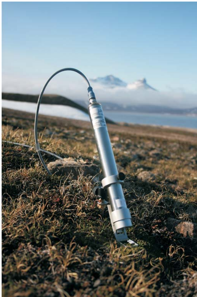
Fig. 4. Measuring head of the fluorometric system Moni-PAM (Walz, Germany).
