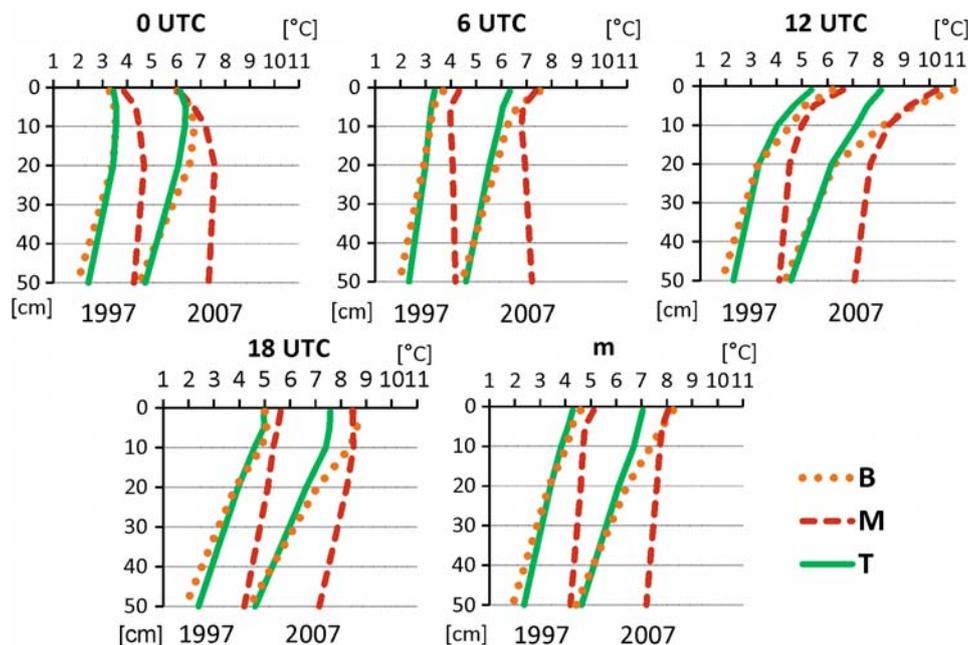
Fig. 8. Mean seasonal vertical ground temperature profiles in the 1–50 cm layer in the three analysed ecotypes (B – Beach, M – Moraine, and T – Tundra) on the Kaffiøyra Plain at selected hours (0, 6, 12 and 18 UTC) and for the daily mean (m) in the warmest (2007) and coldest (1997) according to the ground thermals summer seasons.
