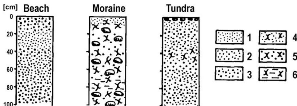
Fig. 3. Ground structure of the ecotopes (Beach, Moraine and Tundra) where ground temperature was measured. Key: 1 – fine sand, 2 – medium-grain sand, 3 – sand gravel, 4 – sand till, 5 – gravel till, 6 – silt till. (Source: Wójcik and Marciniak 1987).
