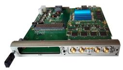
Fig. 5. AMC carrier with FMC connectors together with high speed ADC FMC card developed and shared on OHL license [9]
