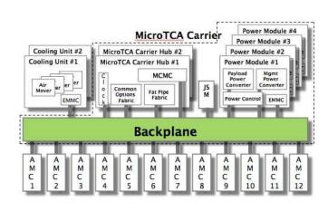
Fig. 2. Example MTCA architecture [?]
