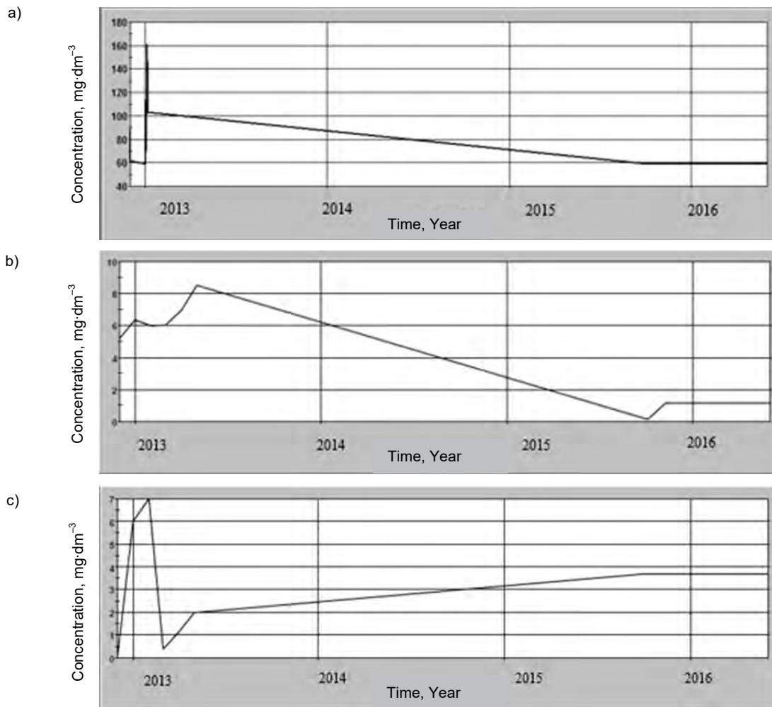
Fig. 6. Simulation of concentration measured and calculated by WASP: a) CBOD1U, b) DO, c) nitrate ( $\text{NO}_3$ ); source: own study
