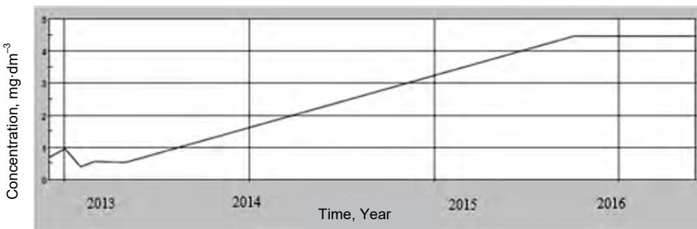
Fig. 7. Simulation of orthophosphate ( $\text{OPO}_4$ ) by WASP measured and calculated with WASP; source: own study
