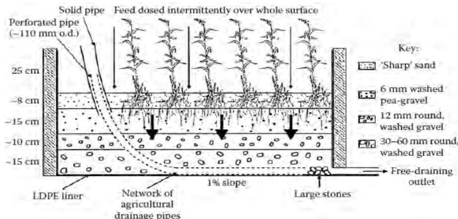
Fig. 14. Vertical flow wetland; source: KADLEC and WALLACE [2009], modified
