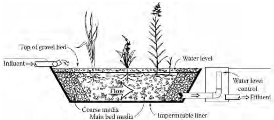
Fig. 12. Deep flow wetland; source: KADLEC and WALLACE [2009] adapted by Ajeagah *et al*
