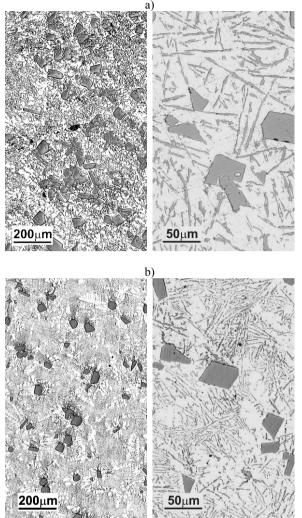
Fig. 8. Microstructure of AlSi19 alloy poured without cooling of probe (a) and with water mist cooling of metalic probe (b). Phase  $\beta$  (Si), lamellar eutectic  $\alpha+\beta$  (Al+Si)
