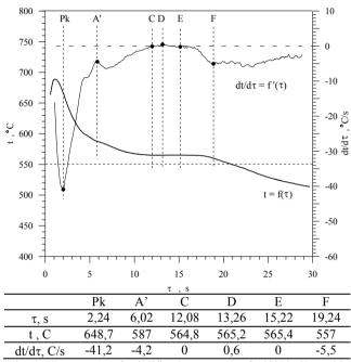
Fig. 6. TDA curves of solidification process of AlSi19 alloy with water mist cooling obtained by thermographic method
