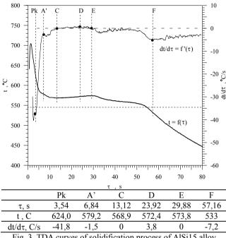
Fig. 3. TDA curves of solidification process of AlSi15 alloy without cooling obtained by thermographic method
