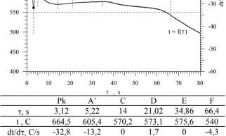
Fig. 5. TDA curves of solidification process of AlSi19 alloy without cooling obtained by thermographic method
