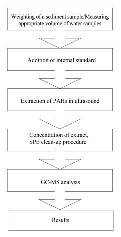
Fig. 2. A diagram of the procedure of PAHs determination in water and sediment samples by GC-MS method
