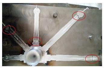
Fig. 8. Hot tears in AlCu4Ti alloys
