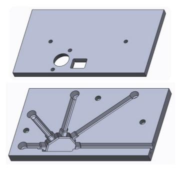
Fig. 3. Final mold design
