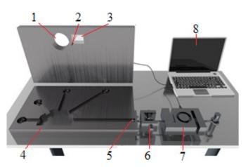
Fig. 5. Measuring apparatus (1 – Inlet, 2 – Thermocouple, 3 – Refractory glass, 4 – Mold, 5 – Anchoring screw, 6 – Gripping mechanism, 7 – Load cell, 8 – Data processing unit)
