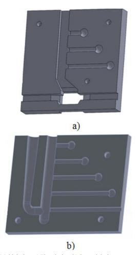
Fig. 1. Mold design: a) First design, b) Second design
