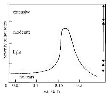
Fig. 10. Hot tears extension depending on Ti amount [7]
