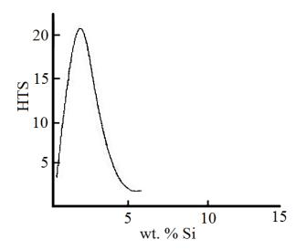
Fig. 7. Hot tears extension depending on Si amount [5]
