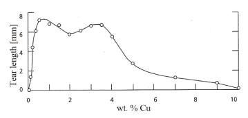
Fig. 9. Hot tears extension depending on Cu amount [6]
