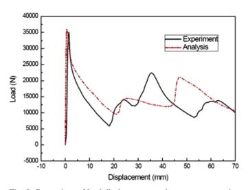
Fig. 5. Comparison of load-displacement graph among compression experiment in case 3 with aluminum foam
